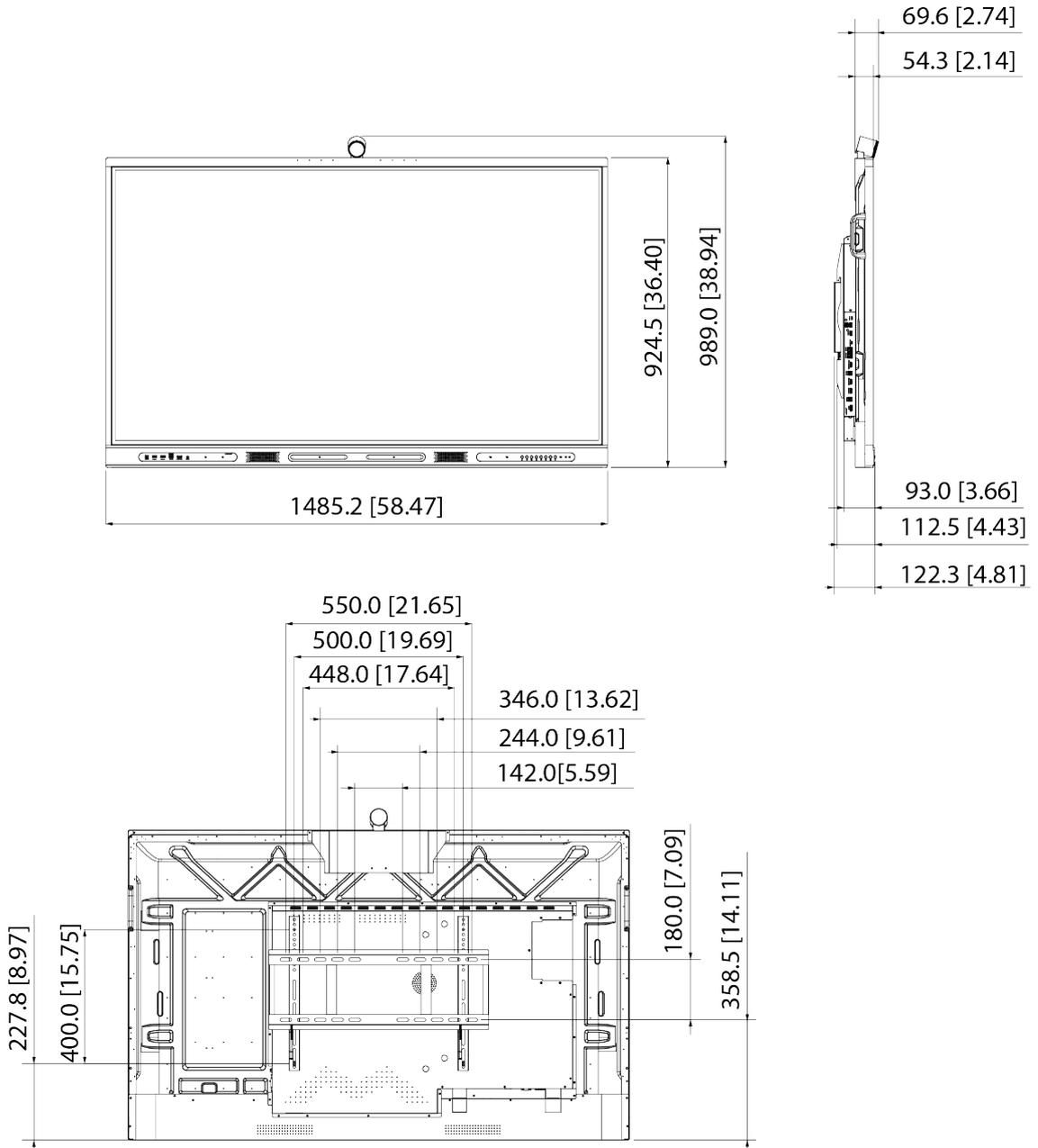
Figure 1-4 Dimensions (without camera) (mm [inch])
