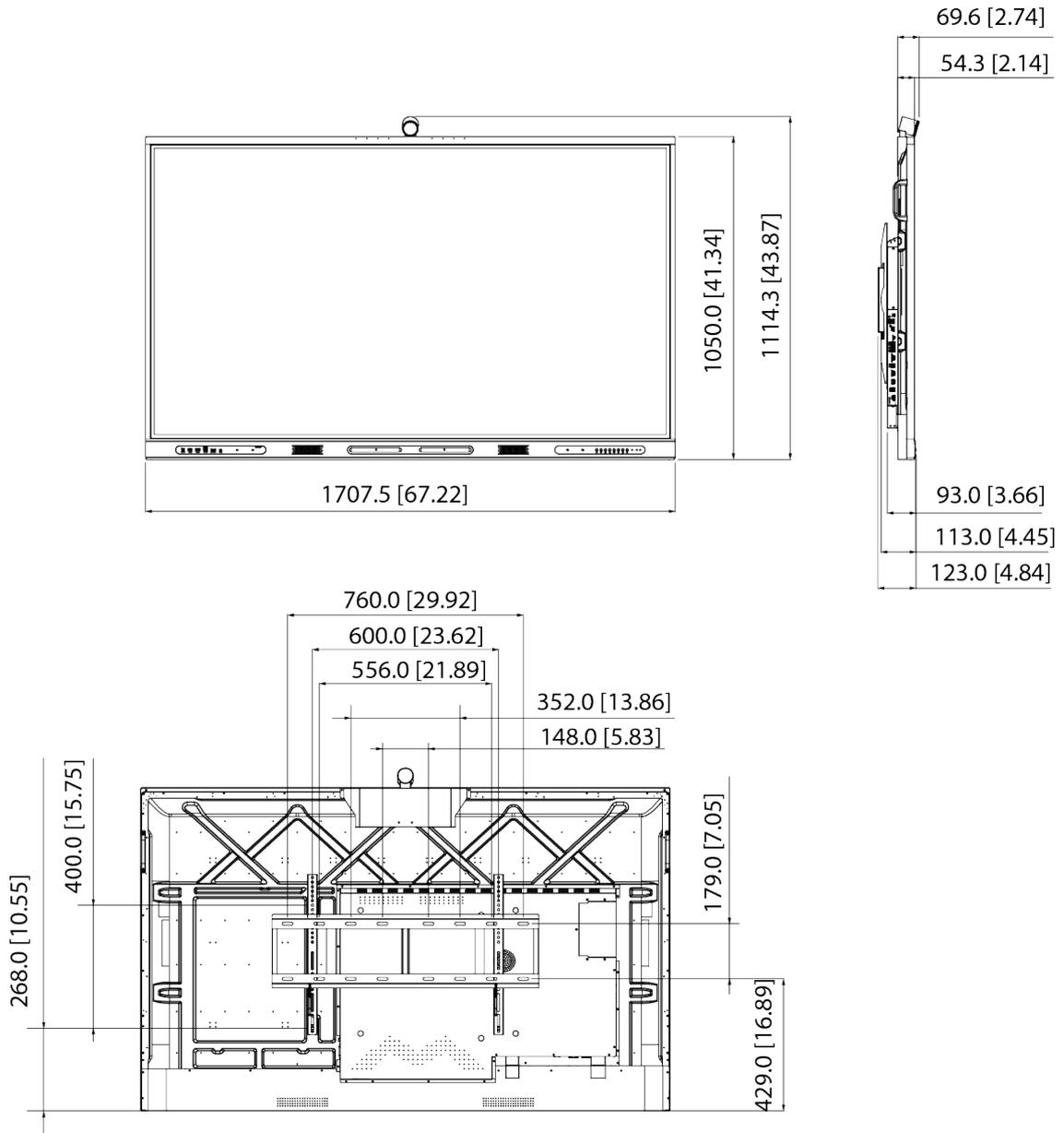
Figure 1-6 Dimensions (without camera) (mm[inch])
